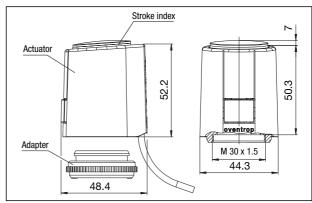
Dimensions actuators with connection thread M 30 x 1.5
