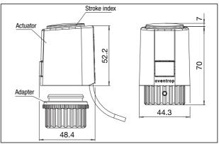
Dimensions actuators with squeeze connection
