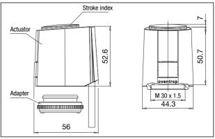
Dimension actuator with auxiliary switch
